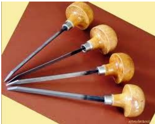
Fig. 1 Gravers and burins
