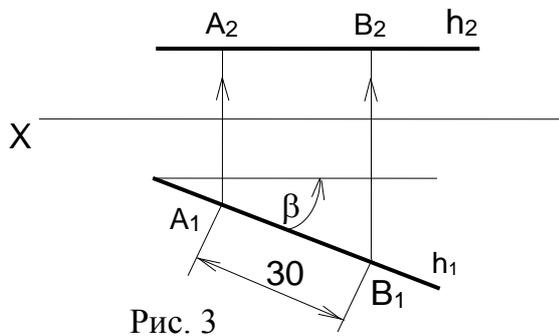
$$h_2 \parallel X, h_1 \not\parallel X$$
