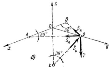
$$\begin{aligned}\sum X &= S_B \cos 60^\circ - S_A \cos 60^\circ = 0 \\ \sum Y &= -(S_A + S_B) \cos 30^\circ + S_C \cos 60^\circ = 0 \\ \sum Z &= -T + S_C \cos 30^\circ = 0\end{aligned}$$
