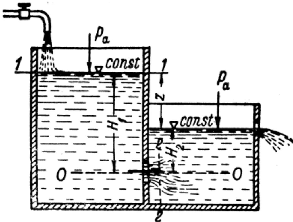
$$H_1 + \frac{p_a}{\gamma} + \frac{\alpha_1 v_1^2}{2g} = H_2 + \frac{p_a}{\gamma} + \frac{\alpha_2 v_2^2}{2g} + h_{1-2}$$
